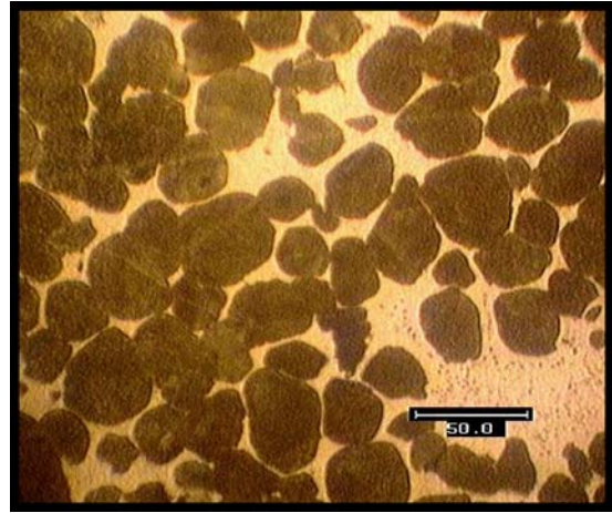
Figure 9 microphotograph of 70%Co-Cu sample processed for 2.5 min.
